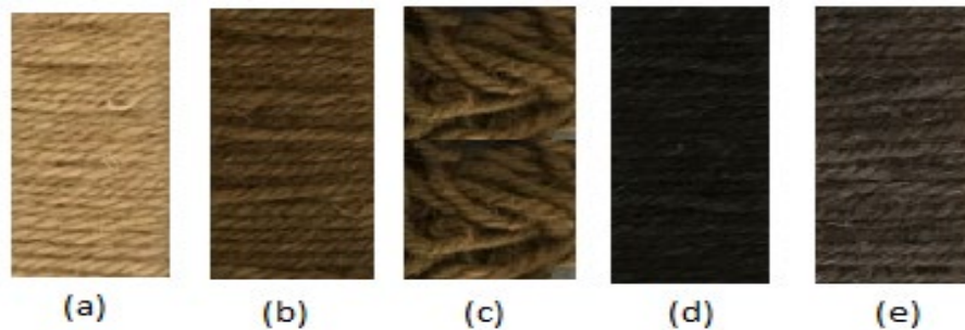
Figure 1. Tetra leaf dyed threads a) Without mordant b) With %3 CuSO 4 Mordant c) With %5 CuSO 4 Mordant d) With %3 FeSO 4 Mordant e) With %3 FeSO 4 Mordant
